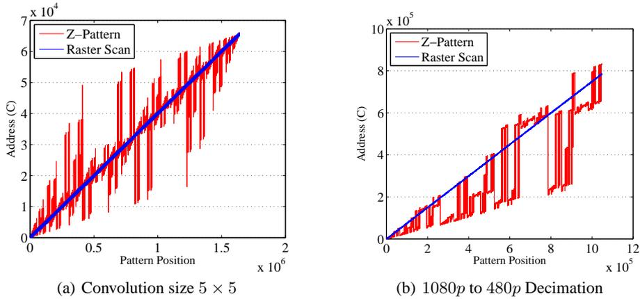
**Fig. 7.** On-chip memory access (C) performance for decimation and 2D convolution for a model with one PE and one execution thread. Output frame size is  $256 \times 256$  pixels.
