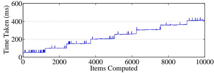
Fig. 5. Concurrent Thread Estimation for the nVidia GeForce 7900 GTX (1300 per batch)
