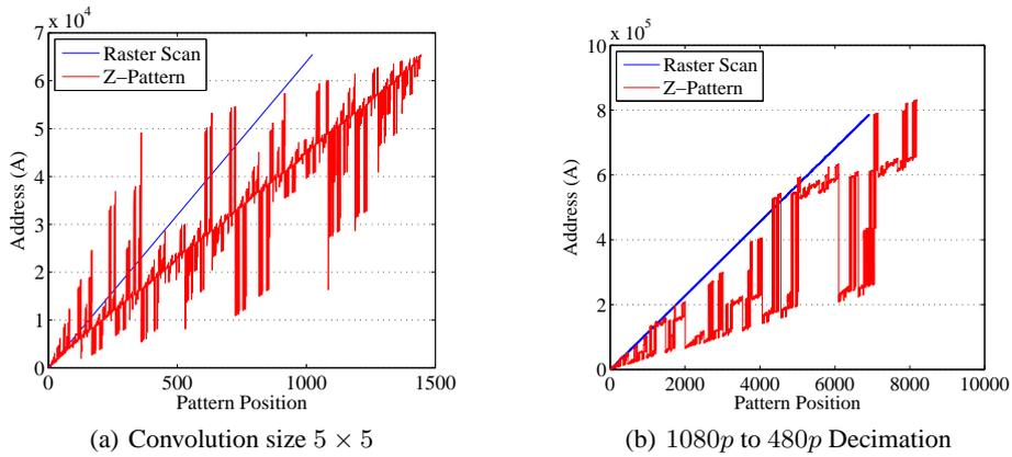
**Fig. 8.** Off-chip memory access ( $A$ ) performance for decimation and 2D convolution for a model with one PE and one execution thread. Output frame size is  $256 \times 256$  pixels.
