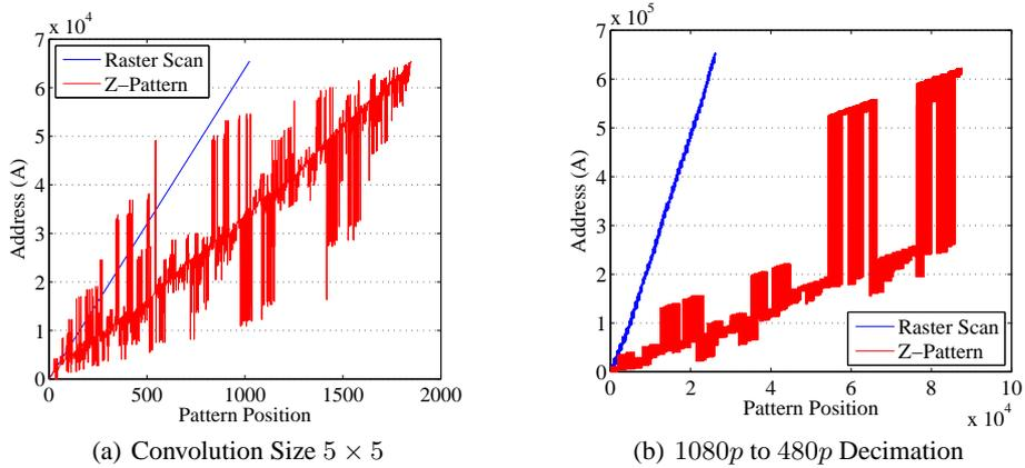
**Fig. 9.** Off-chip memory access ( $A$ ) performance for a model with sixteen PEs and  $\hat{T} = 1500$  (equivalent to nVidia GeForce 6800 GT). For an output frame size of  $256 \times 256$  pixels.
