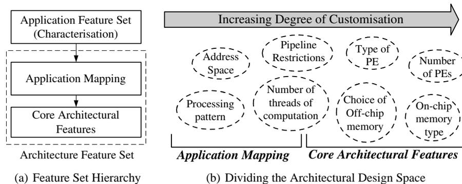
**Fig. 3.** The Architectural Design Space for the HoMP Class of Architectures
