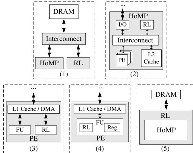
Key: I/O is the input/output interface, FU is the functional unit of a processing element (PE), RL is reconfigurable logic and Reg is a set of local register files
