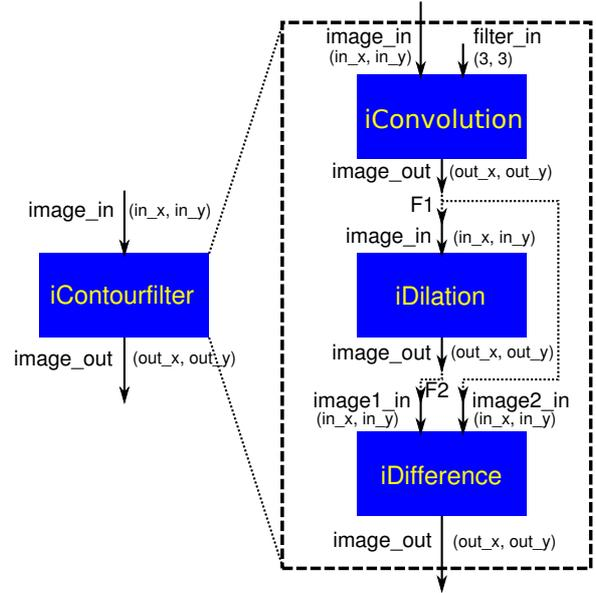
**Fig. 1.** A contour filter example showing dependencies, data flows and size descriptions of inputs and outputs.
