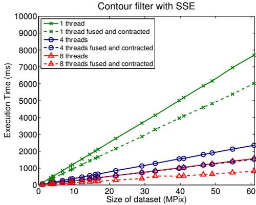
Fig. 6. Execution time of the contour filter example.
