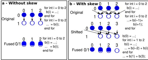
Fig. 4. A simplified one-dimensional loop fusion example.
