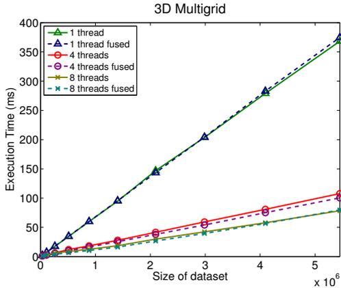
**Fig. 8.** Execution time for single and four and eight threaded 3D multigrid solver kernel.
