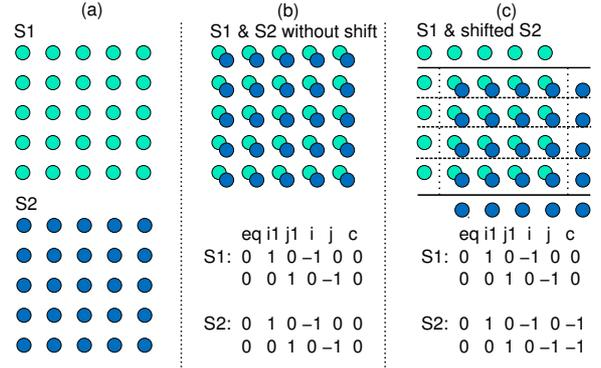
Fig. 5. The scatter matrix can be used to schedule the loop by changing the logical execution time of a given iteration.
