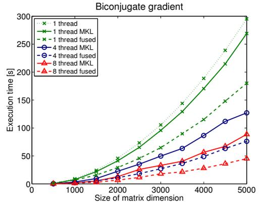
Fig. 7. Comparing MKL, with custom version of biconjugate gradient for 1, 4 and 8 threads (custom without fusion shown only for 1 thread).
